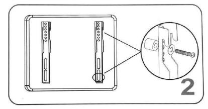
With the strips fitted to the back of your screen, hook into place along your wall. Insert the long screws near the bottom to secure in place.
