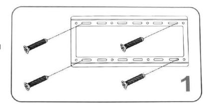
Take the two metal strips provided and screw them onto the back of the AV Screen. Ensure the screw placements are evenly wide apart. Use washers for a secure fit.
